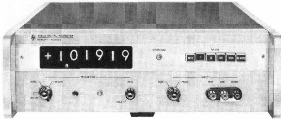
Fig. 6. —hp— Model 3460A Digital Voltmeter has 5-digit resolution but includes 6th digit to permit display of 20% overranging. Input may be through banana-plug jacks on front panel or through guarded connector on rear panel. Measurements are initiated automatically at repetitive rates selectable between 3 per second to 1 per 5 seconds, or singly by front panel pushbutton, or by remote control. Measurement ranges may be selected manually, automatically, or by remote control.
